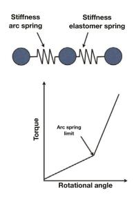
With increasing rotational angle, after the arc spring limits have been reached, the stiffness of the elastomer takes over the work.
